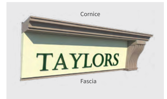
Cornice and Fascia
